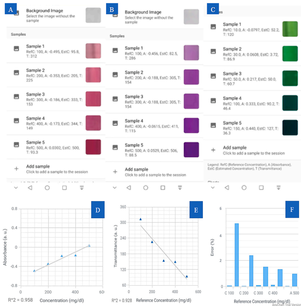
Fig. 5. Samples of calculations using the colorimetric sensing application (A) glucose sample list (B) triglycerides sample list (C) urea sample list (D) calculations of absorbance (E) transmittance (F) error of measurements.
